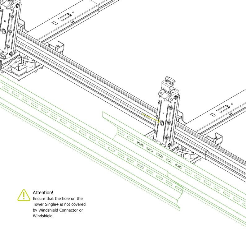
The Windshield Connector is mounted in the same way as the Windshield. Ensure that both components have sufficient overlap.
