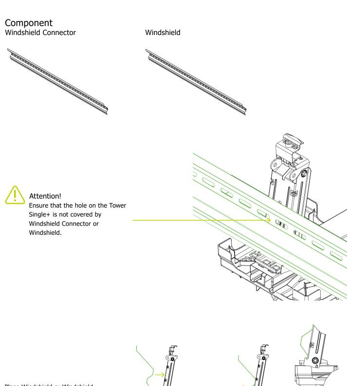
Place Windshield or Windshield Connector on the back of the Tower Single+ and slide it down into the cut-out provided.
