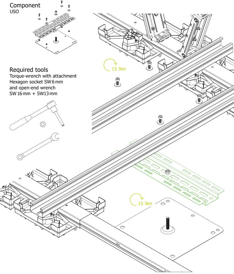
The USO attachment points are located on the Roll-bar or Splice for roll-bar and should be fitted before the USO is assembled. The USO connection should be fixed as close as possible to a rail.
