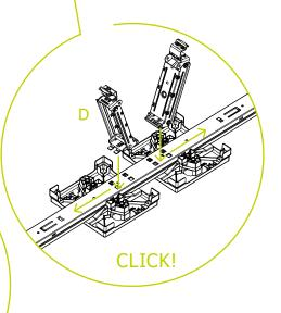
Press the Base Single E with the locking lugs vertically into the recesses of the Ground rail short B and push it towards the middle of the rail until you hear a click. With Ground rail A, the Base Single E must be placed with the locking lugs pointing away from the centre of the rail and locked in place.
