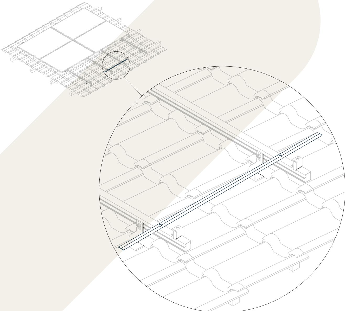
The mounting rails can be connected to each other with ground continuity in a single-layer setup using the sflex alubar 3-27-1160 mm. For landscape installation, the connection is made between the module columns; for portrait installation, between the module rows.
